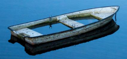
Vessels with level flotation have buoyancy installed to national standards high up in the extremities, allowing the vessel to float level with the waterline if it becomes swamped or flooded. Whether the vessel capsizes or stays upright, level flotation offers a number of advantages for people who find themselves in this predicament.
