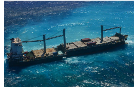
MV Kea Trader, aground with fractured hull (Maritime Cyprus)
