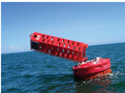
Damage to an AtoN caused by tropical cyclone.
