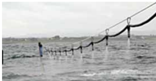
AMOSC boom vane dispersant delivery system
