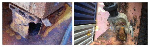
Heavily corroded container securing socket and lashing point
