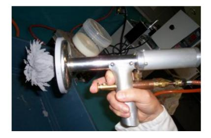
Figure 7: The "third generation" magnetic harvester
