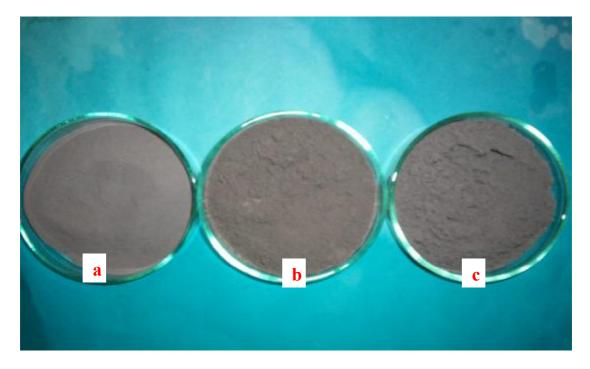
**Figure 66**: (a) Original iron powder; (b) recycled iron powder (from Diesel Oil experiments); (b) recycled iron powder (from Bunker Oil 1 experiments).
