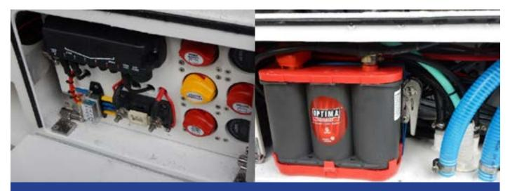
In this example, switch gear and trim tab controls are located within the same compartment as the batteries, causing a risk of explosion. The electrical components were subsequently relocated out of the battery compartment and the batteries were placed into battery boxes. The transom area has since been redesigned by this manufacturer to provide a dedicated battery compartment, removing the source of ignition (engine wiring) from the battery.
