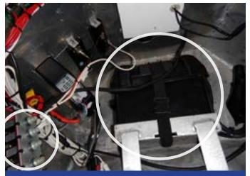
In this photo the battery is contained within a battery box, which is secured with the terminals covered. Ventilation is the key issue — the battery box is not sealed with external ventilation so if for some reason the battery vents it will discharge volatile gasses within a confined enclosure that contains numerous sources of ignition.
