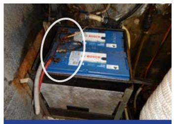
No cover on the battery box means the terminals are exposed and the possibility of the battery shorting out is high, which could lead to a battery explosion or a vessel fire.
