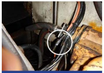
Repairing wires with tape is not considered adequate protection. The connection should be contained within a junction box.
