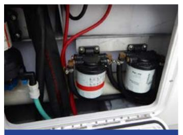
Here, large unsupported wiring is seen running next to fuel filters. Above these filters is a capstan winch, which is a source of ignition and could have ignited the filters and caused an explosion. The filters were subsequently relocated into a compartment that was free of an ignition source.
