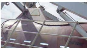
Freefall life boat - Poor condition of high vis paint and windows opaqueSpace Entry
