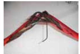
Damaged push-pull cable of lifeboat on-load release gear
