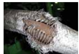
Main engine high pressure fuel lines damaged jacket pipe
