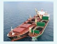
boom were placed adjacent to the grounded *Shen Neng 1*, as an important pollution prevention measure before oil could be pumped off the ship. In the prevailing weather, external oil transfer was a difficult and complex operation and the safety of all concerned was of the highest priority.
