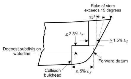
Figure 8 — Requirements for steps in collision bulkheads
