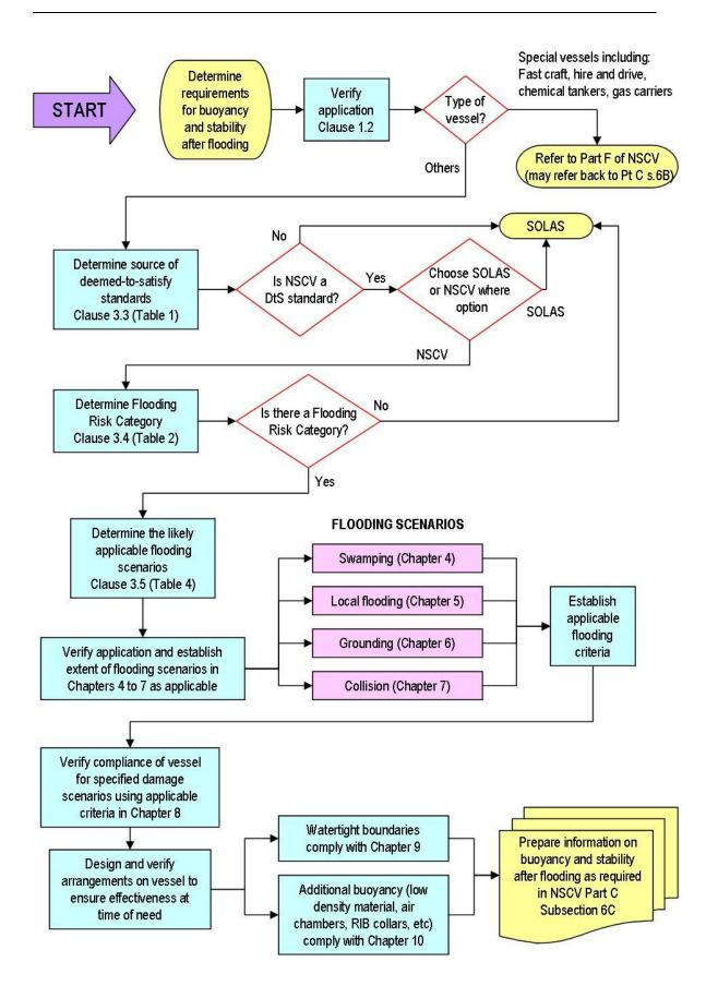
Figure 1 — Flowchart illustrating the use of Subsection 6B
