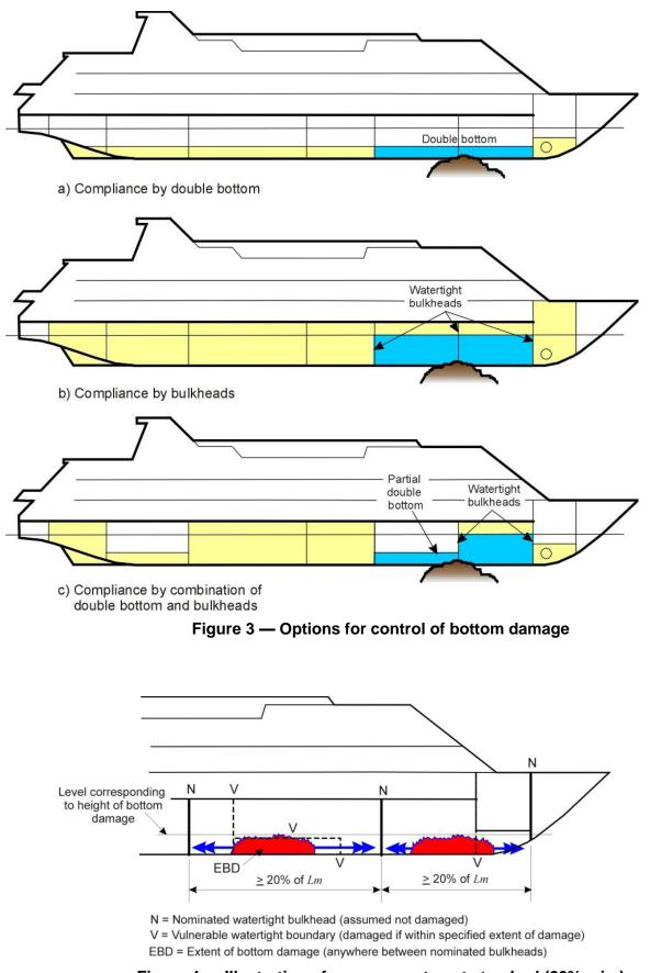
Figure 4 — Illustration of one-compartment standard (20% min.)
