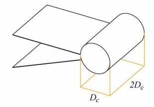
Figure 12 — Assumed panel dimensions for determining the design pressure *P*
