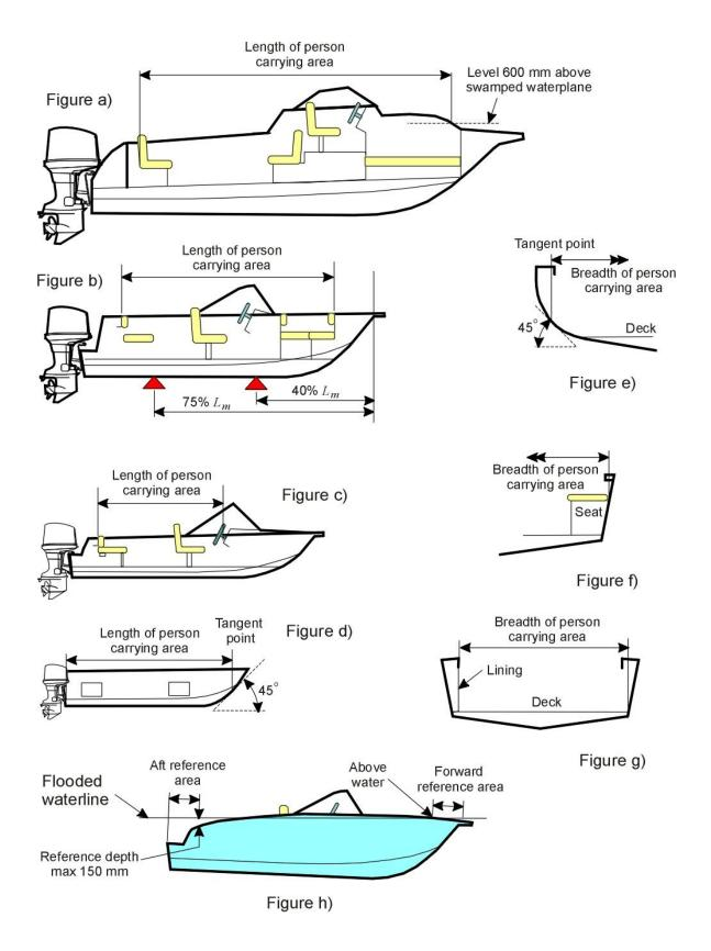
Figure 11 —Illustrations for level flotation criteria
