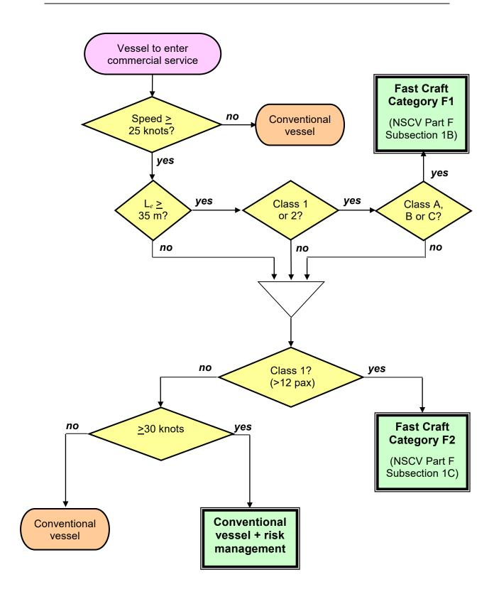
Figure 1 — Flowchart for determining the category of Fast Craft
