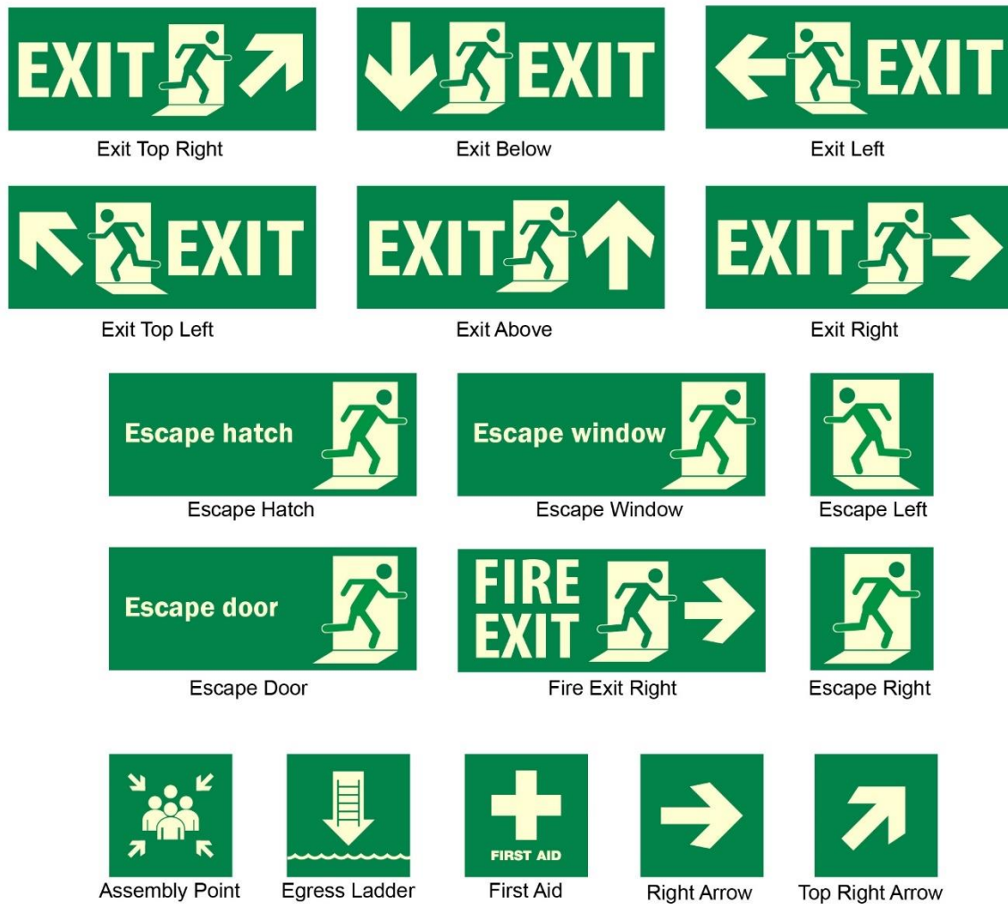
Figure B1 Exit and escape signs
