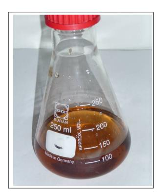
Step 10: Mixture C – dispersed oil suspended in solvent with consistent colour.
